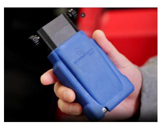
The PUMA line of mobile reflash hardware facilitates quick, easy vehicle reflashing via the vehicle's OBD port.
